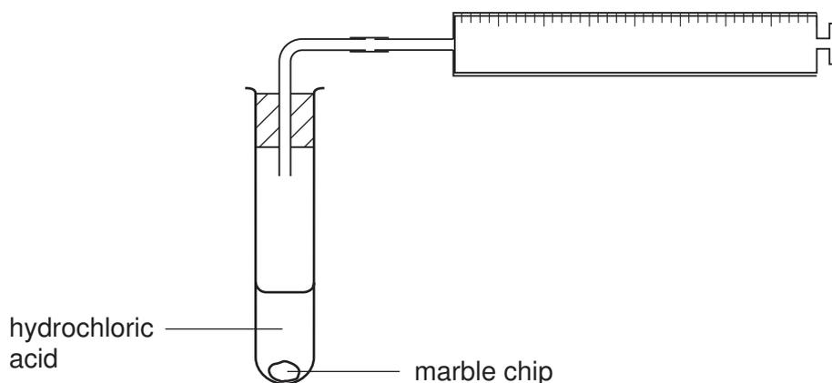
5 test-tubes were put in a rack. To each test-tube was added 10 cm<sup>3</sup> of different solutions of aqueous hydrochloric acid and a marble chip. The marble chips were the same size.
